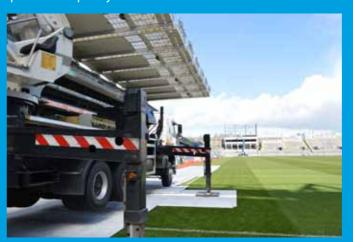
The large 440kg basket capacity on the 50m Bronto Truck Mount meant that the customer could bring more screens on each elevation saving time.
